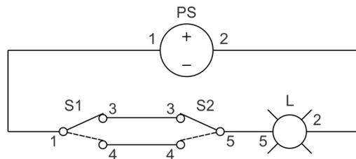
Schematic diagram of a circuit made of a power source and two three-way switches controlling a lamp.
