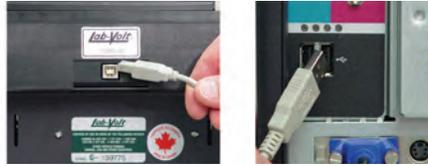
Attach USB Cable to FACET Base Unit and to Computer
