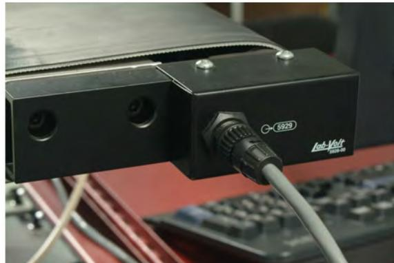
Figure 32. Conveyor Optical Encoder.
