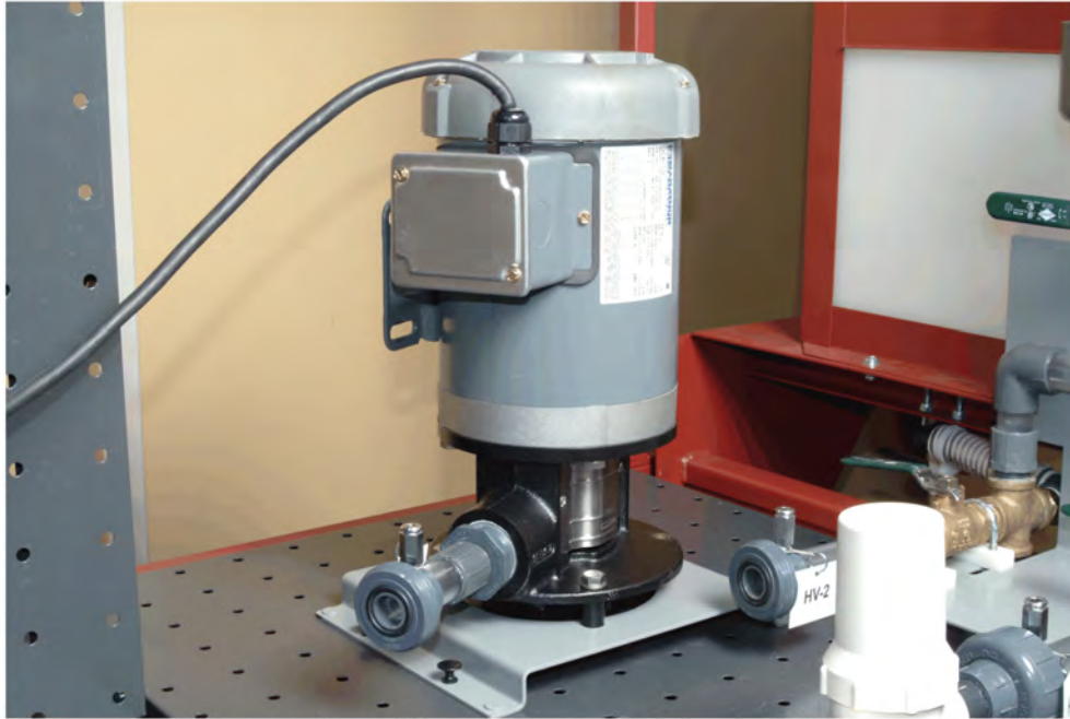
Figure 1-6. Installation of the Multi-Stage Vertical Centrifugal Pump on the pump bench.
