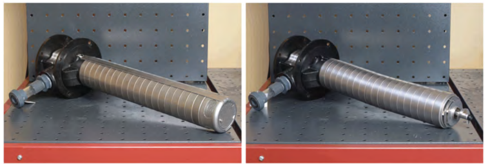
Figure 1-1. Multi-Stage Vertical Centrifugal Pump with suction chamber.
