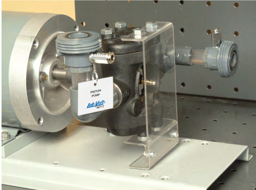
Figure 1-4. Installation of the Piston Pump on the Pump Universal Base.
