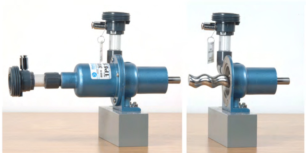
Figure 1-1. Progressive Cavity Pump with and without stator.
