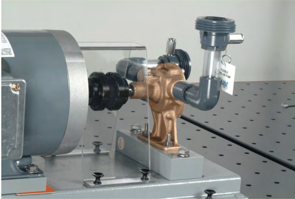
Figure 1-4. Installation of the Flexible Impeller Pump on the Pump Universal Base.
