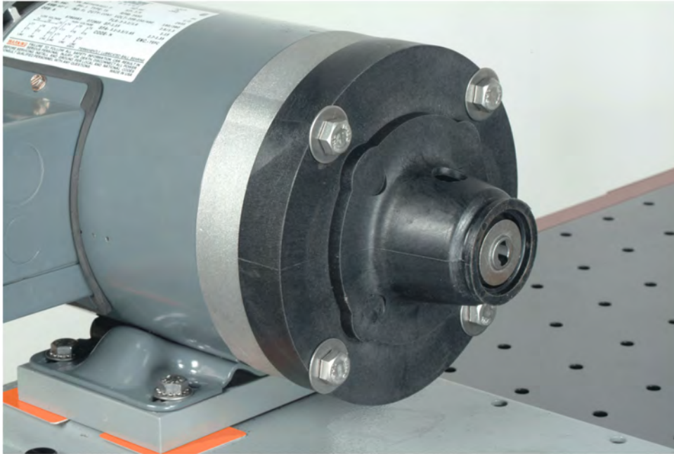
Figure 1-8. Attach the motor adaptor to the Motor.
