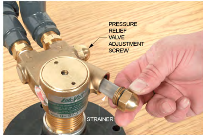
Figure 1-3. A built-in relief valve protects the pump and its piping from over pressurization.
