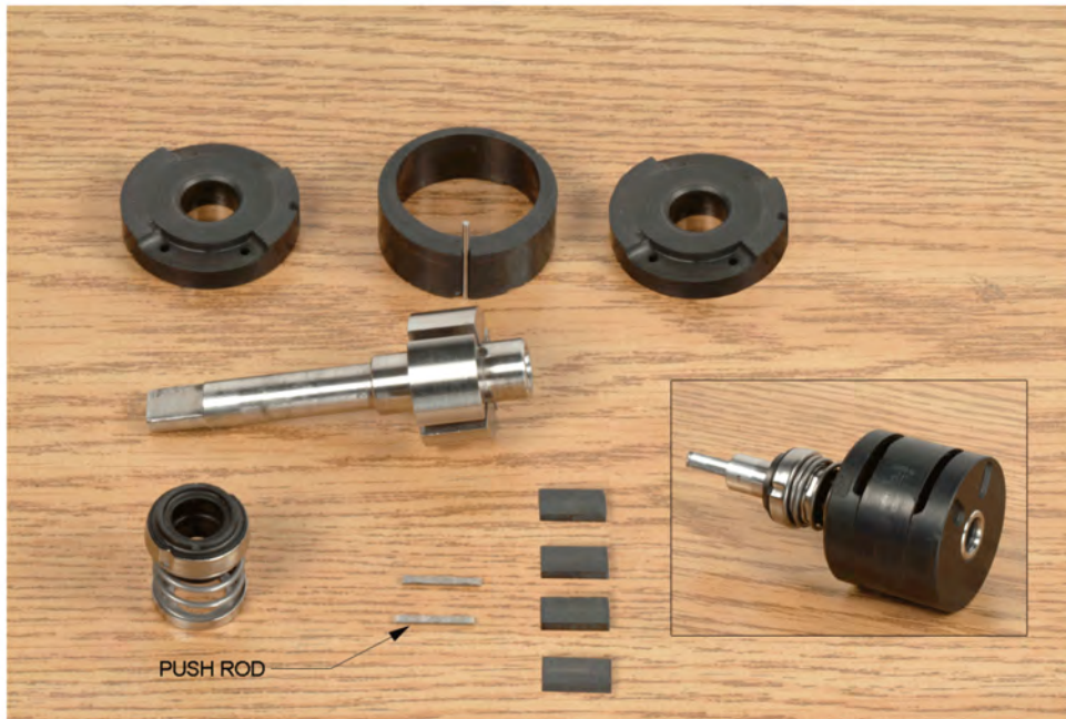
Figure 1-6. Components of the rotor assembly.
