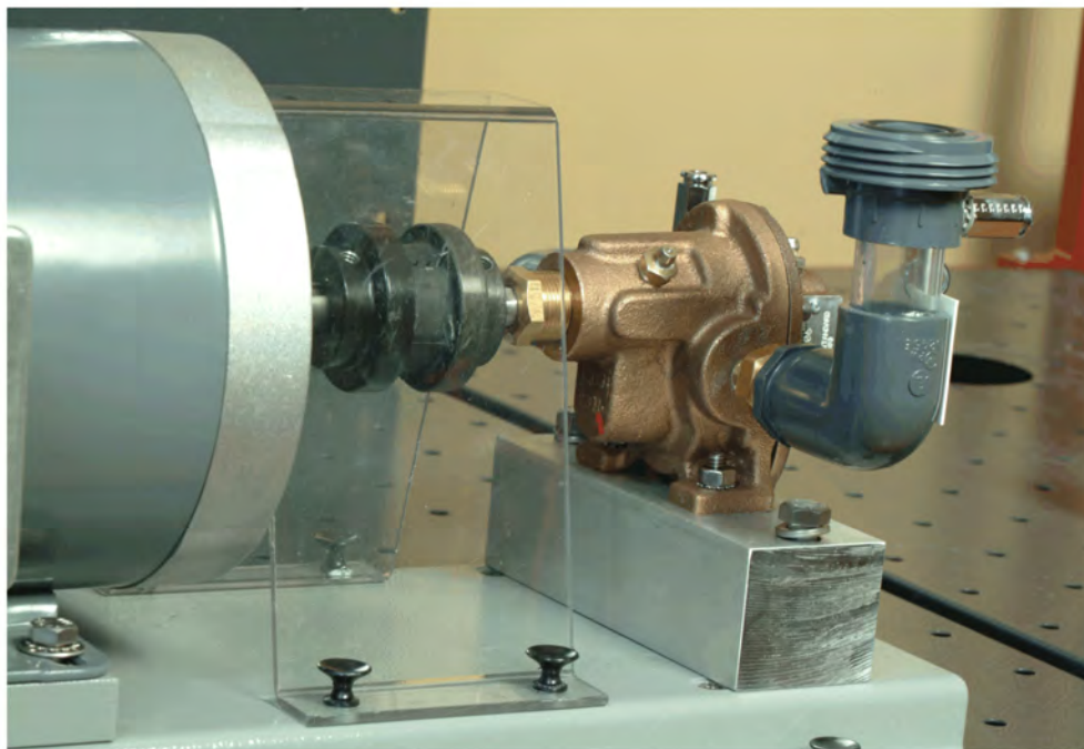
Figure 1-4. Installation of the External Gear Pump on the Pump Universal Base.
