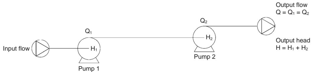
**Figure 4. The discharge line of one pump is connected to the suction line of the other pump.**
