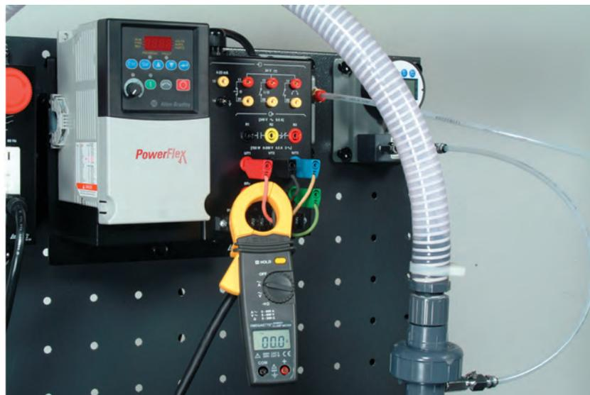
Figure 35. Measuring the current using a Current Clamp Meter.
