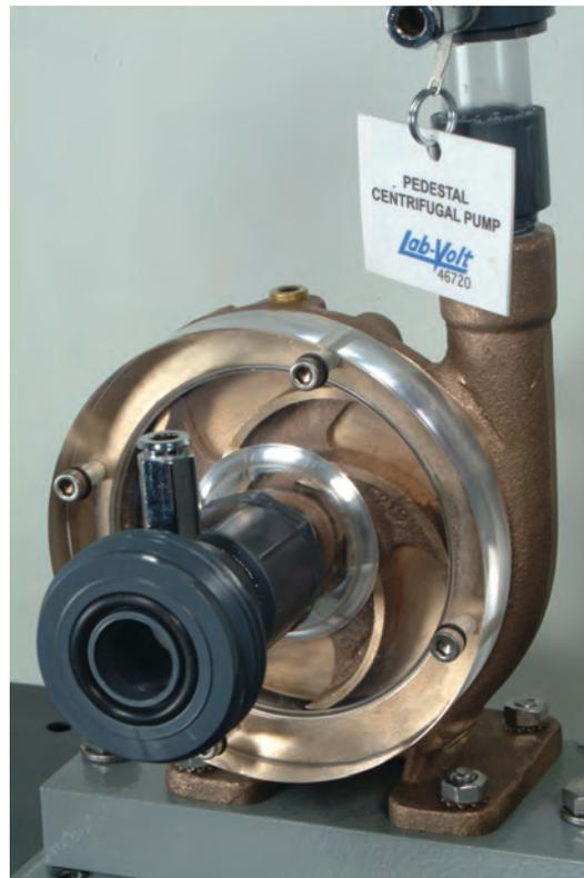
Figure 33. Centrifugal Pump with transparent cover.
