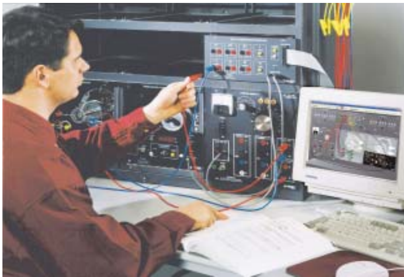
The simulation features of LVSIM-EMS (above) and the modern and versatile instruments of LVDAM-EMS give trainees a virtual hands-on experience before using the actual equipment, saving lab time and equipment costs while enhancing learning.
